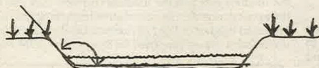
Figure 2. Overwidened stream channel has a bank angle greater than 90 degrees.
