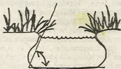
Figure 1. Narrow, deep stream channel has a bank angle less than 90 degrees.
